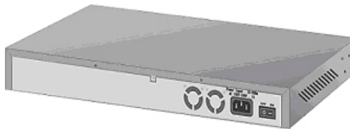
Figure 2-3. The Rear Panel of the LevelOne GSW-2490TXM SNMP Switch
